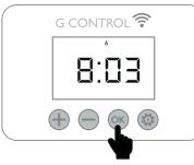
4. Again using the 🕂 and 😑 buttons you can modify the hour and press 🐼 button to confirm and move to minutes.
