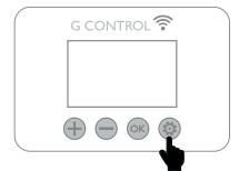
3. Using 🕀 or 😑 buttons scroll until the time is displayed and press 💿 button
