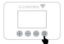
3. Using 🕂 or 🛑 buttons scroll through the menu until "PArA" is displayed on the screen and press 🙉
